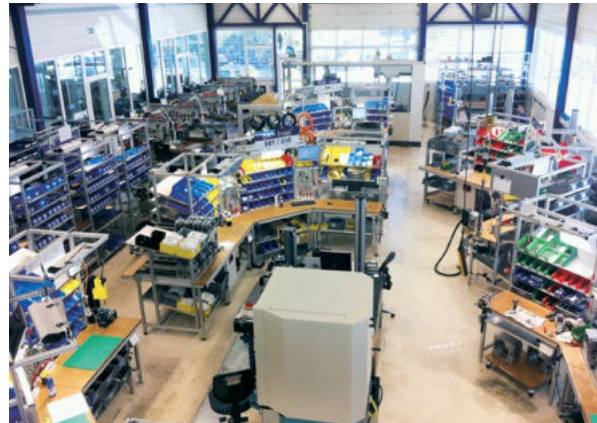
Assembly area with Kanban System
