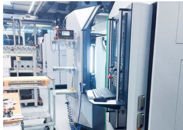
High precision circular and flat grinding
